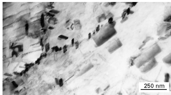
Figure 11 TEM micrograph showing bimodal distribution of VN precipitates at 860 °C annealed for 6 h.
