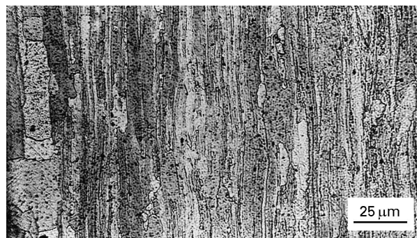
Figure 2 Micrograph showing partially recrystallized microstructure ( X \approx 0.2) of the specimen annealed in hydrogen atmosphere at 820 °C for 500 h.
